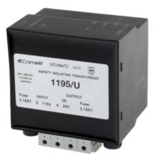
All systems. Transformer with 115VAC primary. 24VAC / 72 VA secondary. The transformer is fitted with fuse internal protection.
