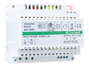
110÷240VAC / 50÷60Hz, 56VDC power supply unit, 100W, with DIN bar (6 modules). Dimensions 99 x 93 x 53 mm.
