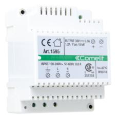
Power supply unit with input of 100÷240VAC/50÷60Hz, 33VDC output with 500mA continuous and 1.2A inrush current for video door entry panel. Equipped with internal protection against overcurrent and short circuits. Dimensions: 71.7x90x62 mm (4 DIN modules).
