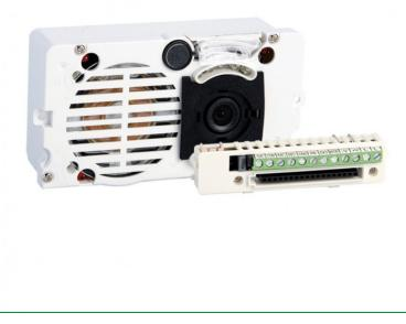
Audio-video unit for ViP system including terminal block complete with front-adjustable mini lens colour camera, LED camera lighting. Complete with terminal block and digital audio management system with Eco-cancelling, watertight loudspeaker and electret microphone, loudspeaker volume adjustable from the front. For fitting in modules: art. 33410, 33411 and 33412. Dimensions: 102x55x38 mm.
