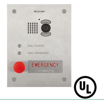
Stainless steel entrance panel with a single call button and indicator LEDs for call forwarded and call answered. Complete with POE audio/video module for ViP system and flush-mounted box. "EMERGENCY" model with Braille text. Can be wall-mounted using accessory Art. 3461. POE entrance panel. Compatible with H.264 video format. Dimensions 229x178x59mm.
