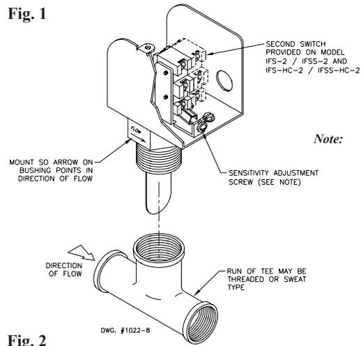
**Note:** Turn screw clockwise to increase the flow rate required to activate the switch. Turn screw counter-clockwise to decrease the flow rate required to activate the switch.
