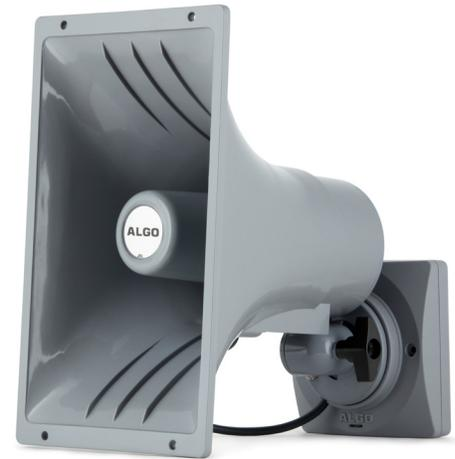
The Algo 8186 IP Horn Speaker is a powerful self-amplified audio communication device capable of producing 116 dB of audio output in noisy environments. The 8186 is constructed with durable material and is wet weather rated (IP66), making it ideal for both indoor and outdoor locations. The hard shell ensures the speaker can withstand impact from debris and exposure to water in extreme weather conditions.
