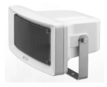
The CS-154U outdoor speaker features stainless steel hardware for all-weather durability. It is designed to offer the high intelligibility of weather-resistant horns combined with the high sound quality of dynamic speakers. The CS-154U employs the rotary switch that facilitates impedance changes. It also employs a constant directivity horn for clear sound output over its horizontal range of 90° operation.
