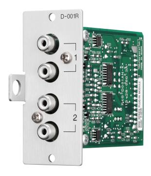
The D-001R is a line input plug-in module designed for use with the 9000 Series amplifiers. It has 2-channel unbalanced inputs of RCA jacks. Input signals to both channels are mixed together. The D-001R can process effect for TONE/EQ/COMPRESSOR to two inputs independently.
