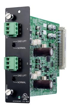
The D-921E is a 2-channel microphone/line input module designed for use with the D-901 Digital Mixer, etc. It is equipped with removable terminal block type connectors. Input sensitivity and phantom power setting can be performed at the main frame such as the D-901.
