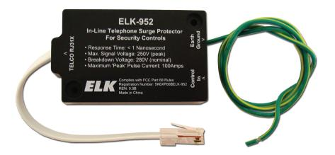
The ELK-952 provides exceptional protection against damage from lightning, voltage spikes, and surge damage coming into a phone line. It installs between the RJ31X Phone Jack and the Security Control. The ELK-952 features multi-stage protection and is 5 times faster than MOVs.
