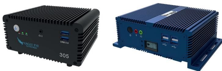
The Eagle Eye Bridge acts as a gateway from your premises to the Eagle Eye Cloud Data Centre where your video is stored and managed by the Eagle Eye Cloud VSaaS. It provides a secure connection, video buffering, bandwidth management, and monitoring of cameras.
