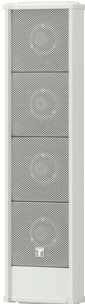
The HA-1030EN is composed of multiple horn speakers positioned in an array. It is a highly efficient speaker. Clear voice can be transmitted to a distant place without acoustic correction. The built-in high-pass filter cuts the bass that can damage the speaker. A double drip-proof structure, and a salt-resistant paint finish, it has excellent durability in an outdoor permanent environment.
