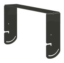
The HY-1200HB Mount Bracket is designed to mount speaker system to a wall or ceiling in a horizontal configuration. It allows the speaker orientation angle to be adjusted from 15° upward to 60° downward when mounted on a wall, and from 0° (horizontal) to 90° downward when mounted to a ceiling.
