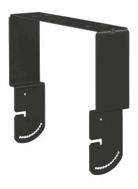
The HY-1200VB Mount Bracket is designed to mount speaker system to a wall or ceiling in a vertical configuration. It allows the speaker orientation angle to be adjusted from 15° upward to 60° downward when mounted on a wall, and from 15° upward to 90° downward when mounted to a ceiling.
