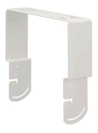
The HY-1200VW Mount Bracket is designed to mount speaker system to a wall or ceiling in a vertical configuration. It allows the speaker orientation angle to be adjusted from 15° upward to 60° downward when mounted on a wall, and from 15° upward to 90° downward when mounted to a ceiling.
