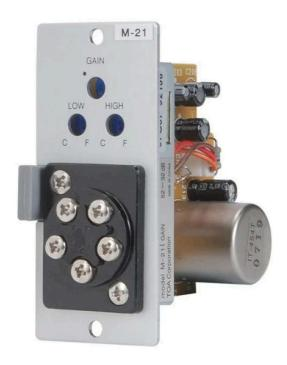
The M-21S is a microphone input module to be used in conjunction with the 900 series components and other TOA's equipment. It has a transformer balanced microphone input with screw terminals, remote volume control function, phantom power supply function, and gain and tone controls.
