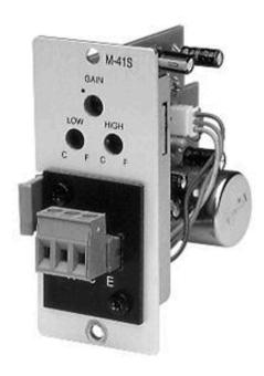
The M-41S is a microphone input module to be used in conjunction with the 900 series components and other TOA's equipment. It has a transformer balanced microphone input with removable terminal block connector, phantom power supply function, and voice-activated muting control output.
