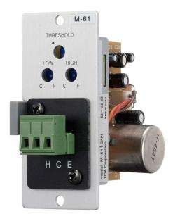
The M-61S is a microphone input module to be used in conjunction with the 900 series components and other TOA's equipment. It has a transformer balanced microphone input with terminal block connector, phantom power supply function, compressor function, and threshold and tone controls.
