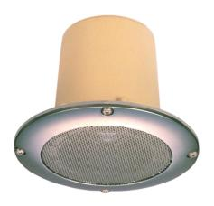
The PC-3CL is a completely-sealed, flush-mounted ceiling speaker made up of a high power handling, splash-proof, small full-range speaker employing a plastic film diaphragm. Its chemical-resistant grille makes the speaker ideal for use in clean rooms, hospital operation rooms, and hot and humid locations such as bath rooms and wet sauna rooms.
