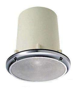
Full-range 8 cm, 2 kohm/5 W speaker with sealed rear chamber, and high-molecular substance speaker vibration section to prevent floating dust particles from contaminating medical, chemical, or IC/photo film production.
