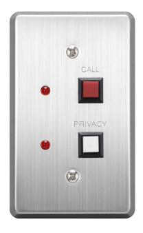
The RS-140 is a switch panel designed for use with the N-8000RS or N-8010RS 2-Core Shielded Substation Interface Unit. It is equipped with a Call button and a Privacy button, and can be installed in a 1-gang electrical box. By connecting a high impedance speaker to it, hands-free conversation with the master station can be made through its speaker. Also, it can be used in connection with the RS-141 Ip Intercom Option Handset.
