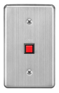
The RS-143 is a switch panel designed for use with the N-8000RS or N-8010RS 2-Core Shielded Substation Interface Unit. It is equipped with a Call button and can be installed in a 1-gang electrical box. By connecting a high impedance speaker to it, hands-free conversation with the master station can be made through its speaker. Also, it can be used in connection with the RS-141 Ip Intercom Option Handset.
