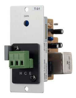
The T-01S is a line output module to be used in conjunction with the 900 series components and other TOA's equipment. It has a transformer balanced line output with removable terminal block connector, and gain control.
