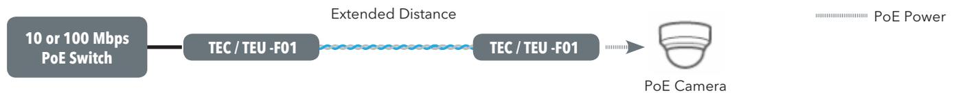
PoE Pass-Through Mode with Multiple Remote Units
