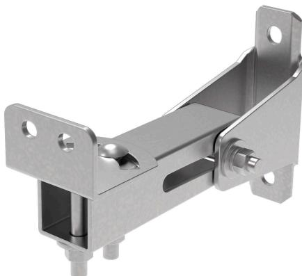
This is a bracket for attaching the HA series Long range array speaker to a wall. The speaker can be adjusted from  $-45^\circ$  to  $+45^\circ$  to the left and right. This bracket comes in one set of 2 pieces.
