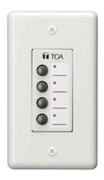
Designed for exclusive use with the 9000M2 Series or M-864D, the ZM-9011 is a wall mounted remote control panel having 4 buttons. It is used in conjunction with the RC-001T Remote control module or M-864D. It can be mounted in a standard 1-gang electrical box in the wall.
