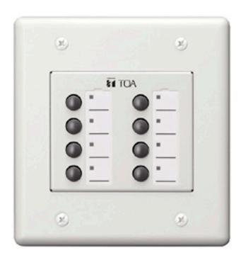
Designed for exclusive use with the 9000M2 Series or M-864D, the ZM-9013 is a wall mounted remote control panel having 8 buttons. It is used in conjunction with the RC-001T Remote control module or M-864D. It can be mounted in a standard 2-gang electrical box in the wall.
