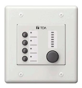
Designed for exclusive use with the 9000M2 Series or M-864D, the ZM-9014 is a wall mounted remote control panel having 4 buttons and 1 volume control knob. It is used in conjunction with the RC-001T Remote control module or M-864D. It can be mounted in a standard 2-gang electrical box in the wall.
