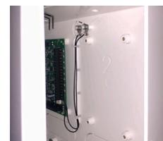
Close, then Open the Door to the enclosure on the IQ Hardwire 16-F. This will "tamper" the module and send a learn in signal to the IQ Panel 2
