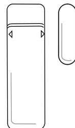
Apply provided adhesive strips to the back of sensor and magnet.
